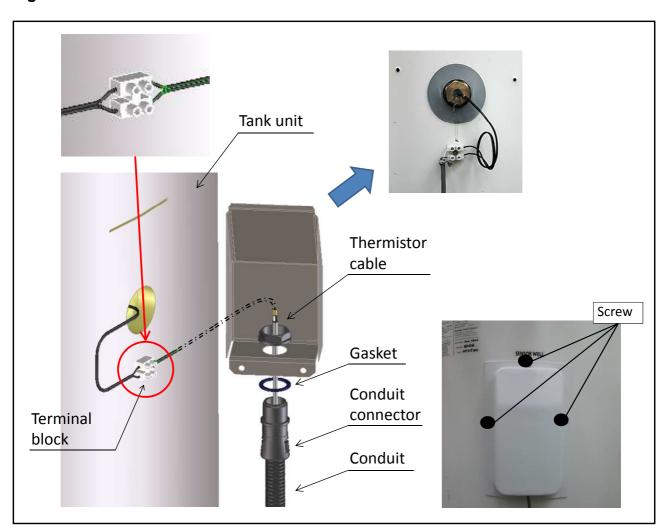
Figure 11: Connect tank unit thermistor cable
