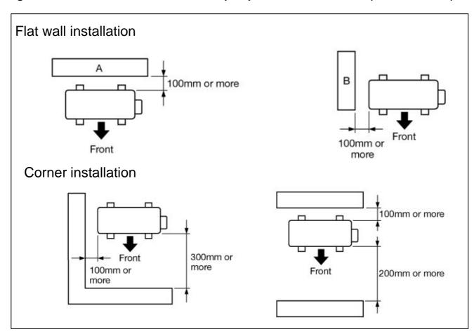
Figure 4: Restrictions on installation with the space between the tank unit and the heat pump unit
