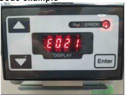
After a component is replaced or the inspection is completed, turn the breaker on/off several times to confirm the error does not re-occur.
