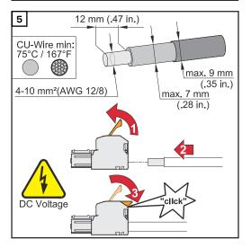
Select the cable cross section in accordance with the instructions in **Permitted cables** from page **61**.
