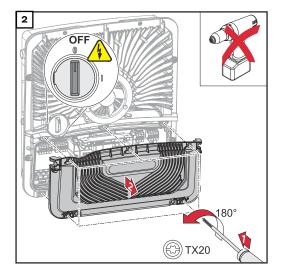
Make sure that the DC disconnector is in the "Off" switch setting.
