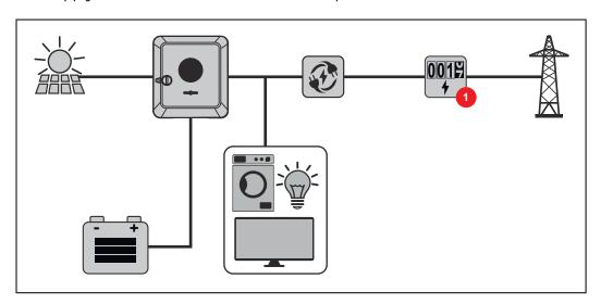
Operating mode – Inverter with battery, Ohmpilot and backup power function
