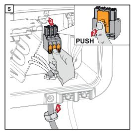
Guide the mains cable through the strain-relief device from below. Remove the OP terminal.
