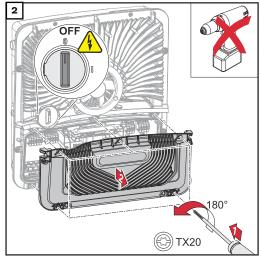
Make sure that the DC disconnector is in the "Off" switch setting.
