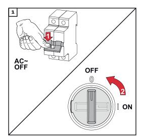
Switch off the automatic circuit breaker and DC disconnector.
