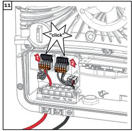
Push the DC push-in terminals into the corresponding slot until there is an audible click.
