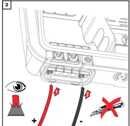
Push the DC cables through the DC bushings by hand.
