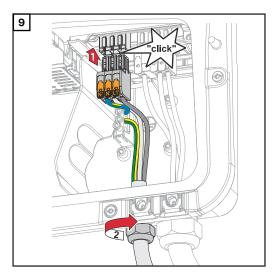
Insert the OP terminal into the OP slot until it engages. Tighten the cap nut of the strain-relief device to the torque specified by the manufacturer.
