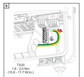
Fasten the battery ground conductor to the second input of the ground electrode terminal from above using a screwdriver (TX20) and a torque of 1.8-2 Nm.
