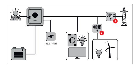
Operating mode - inverter with battery, AC-coupled to another inverter
