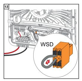
Remove the factory installed bypass on the push-in WSD terminal.
