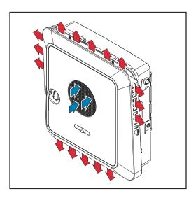
Ambient air is drawn in by the fan on the front side and blown out at the device sides. The even heat dissipation allows several inverters to be installed next to each other.
