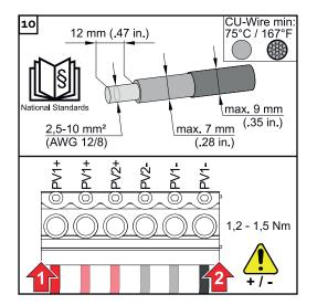
Strip the insulation on the single conductors by 12 mm and secure to the corresponding slot of the terminal on the PC board with a torque of 1.2 - 1.5 Nm.
