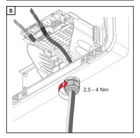
Fasten the cap nut of the strain-relief device with a torque of min. 2.5 - max. 4 Nm.
