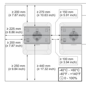
Only install on a solid, non-flammable surface.
