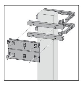
When installing the inverter on a mast or beam, Fronius recommends using the "Pole clamp" (order no. SZ 2584.000) mounting kit from Rittal GmbH.
