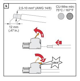
Strip the insulation of the single conductors by 12 mm.
