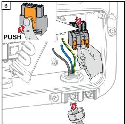
Guide the mains cable from below through the strain-relief device on the right side.
