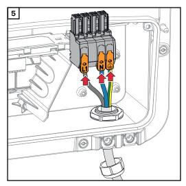
L1 Phase conductorN Neutral conductorPE Ground conductor
