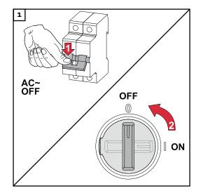
Switch off power to the inverter and wait for the specified time until the capacitors have discharged and the fan has shut down.
