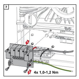
Insert the PC board into the inverter and secure with the four screws (TX20) supplied at a torque of 1.0 - 1.2 Nm.
