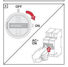
Set the DC disconnector to the "On" switch position. Switch on the automatic circuit breaker.
