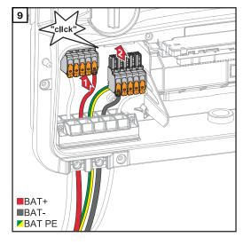
Insert the DC terminals into the respective slot until they engage.
