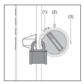
The DC disconnector has three switch settings:
