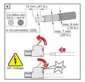
Select the cable cross section in accordance with the instructions in **Permitted cables** from page **61**.
