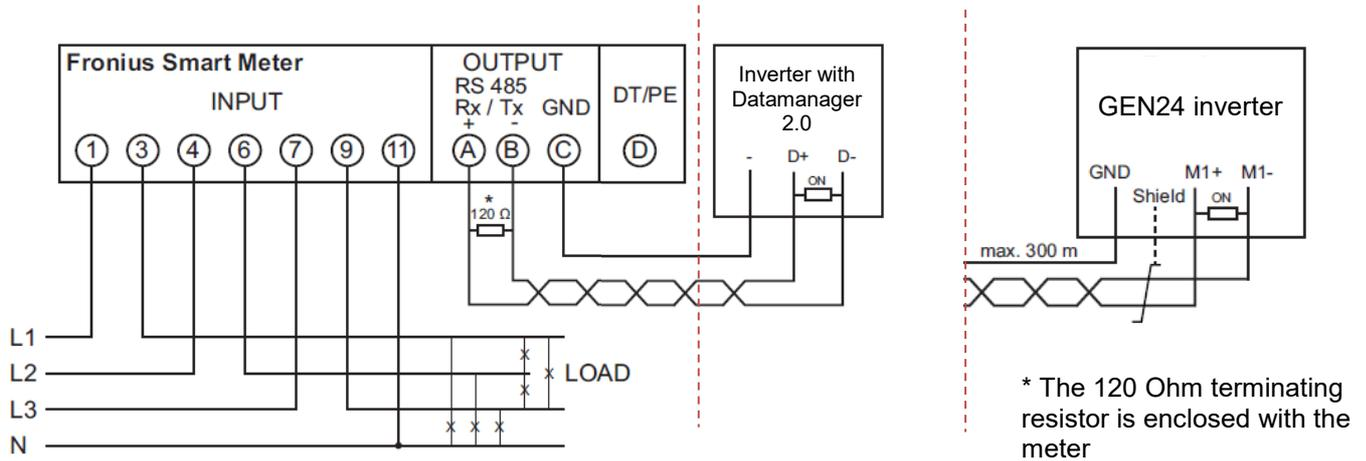
\* The 120 Ohm terminating resistor is enclosed with the meter
