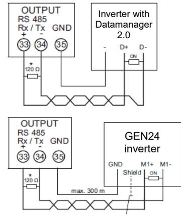
\* The 120 Ohm terminating resistor is enclosed with the meter
