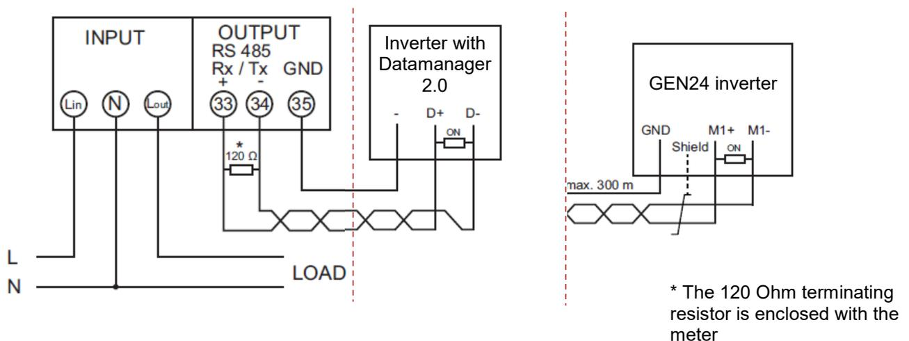
**Wiring detail for Single Phase Fronius Smart Meter TS 100A-1**
