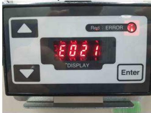
After a component is replaced or the inspection is completed, turn the breaker on/off several times to confirm the error does not re-occur.
